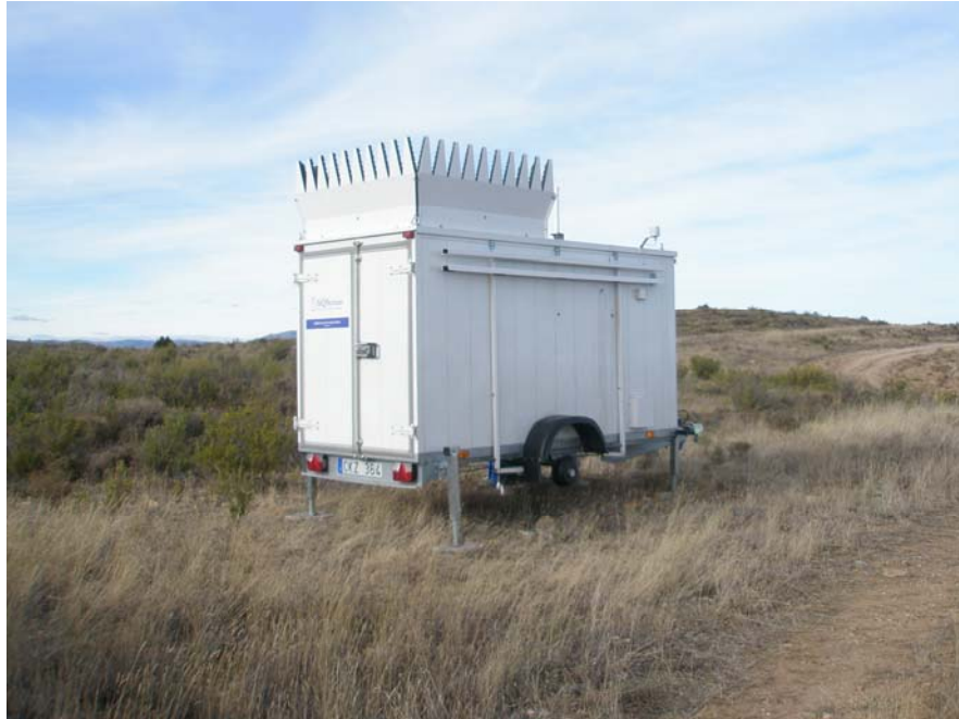
Photograph 1. AQ500 SODAR device.
